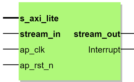
Figure 1. Thermal Color Profile IP Top-Level View
