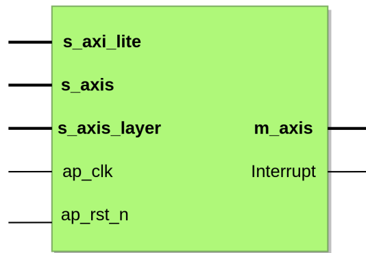
Figure 1. Alpha Blending IP Top-Level View
