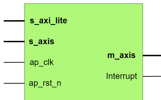
Figure 1. Gamma Correction IP Top-Level View
