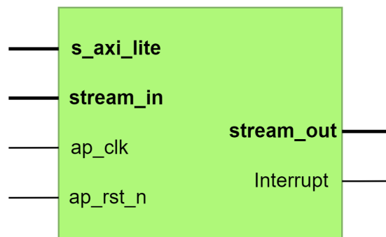
Figure 1. Sharp Enhancement IP Top-Level View
